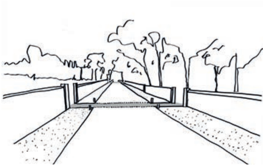
Pedestrian crossing at intervals along the Pales, passing through new openings in the cemetery wall. The crossing would be signified by bollards either side on the verges, and by a high-friction strip across the carriageway in a contrasting material
